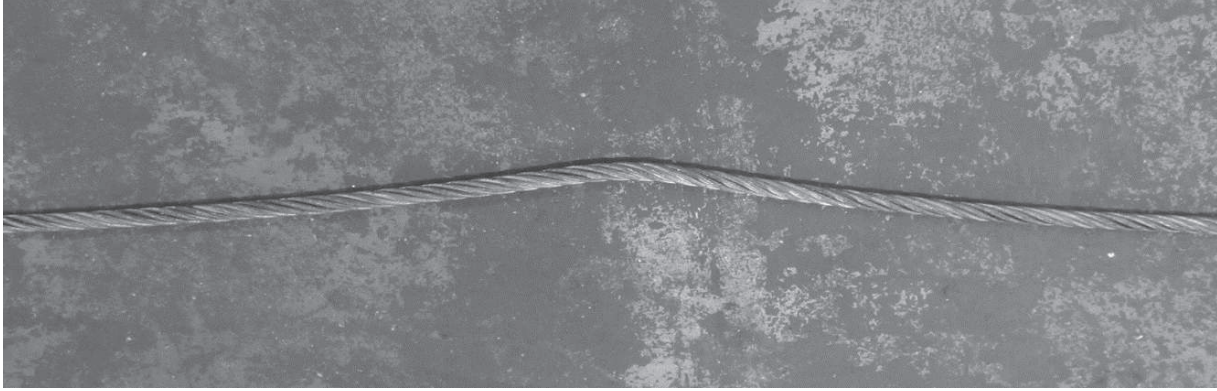
Figure 30-1.8.2-2 Distortion of Rope Structure — Dogleg
