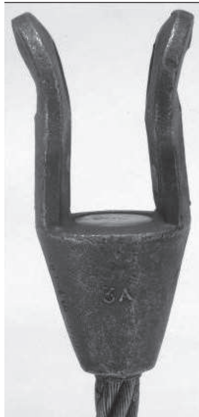
Figure 30-1.8.2-9 Damaged End Terminations
