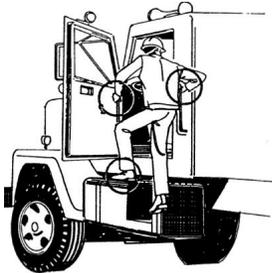
Look at every piece of equipment and large vehicle with the Three Point Rule in mind: contact with the construction equipment or vehicle by either one foot and two hands or one hand and two feet.
