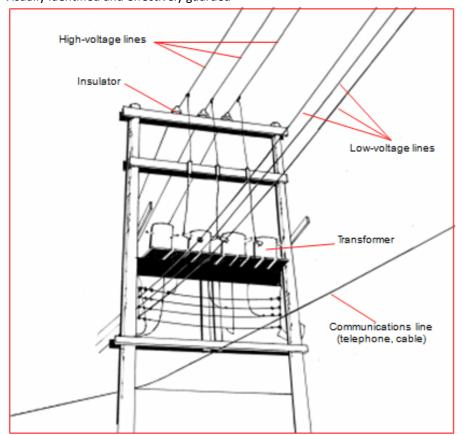
Electricity is transmitted from generating stations and substations via high-voltage transmission lines at 60–500 kV (60,000–500,000 V).
